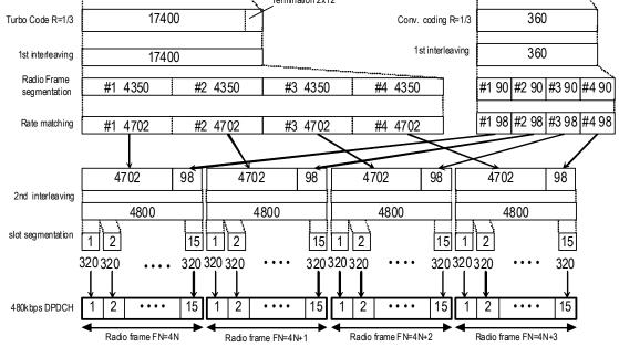
Figure 3.2.2-3 Channel coding for UL reference measurement channel 144 kbps
