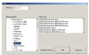
Figure 3.2.9-4 Parameter file reading screen (MG3710A)
