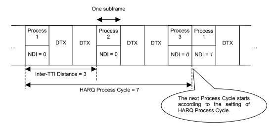
Figure 3.1.4-2 HARQ Process Cycle
