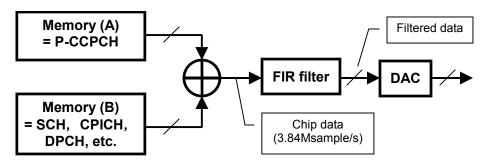
Figure B.1-2 Block Diagram with FIR Filter Used
