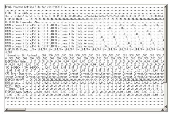
Figure 3.2.4.1-2 Editing HARQ process setting file using text editor
